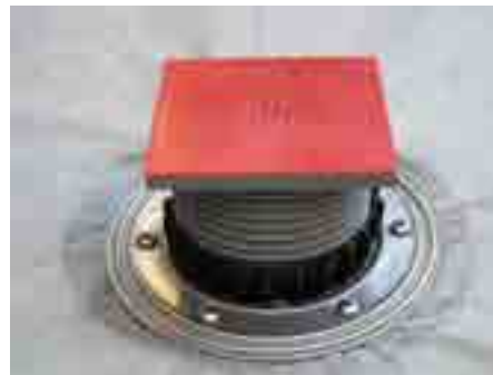
5. Clamp fleece between the stainless steel clamp ring (HL83.0) and the extension (HL85N), set the gravel guard (HL180), adjust the extension to the final slab height
