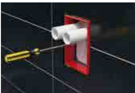
10. When installing a second washing device (or dryer), replace the single cartridge to a double.
